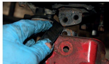
This is why the engine mount has to be undone and pushed into the body bracket – to create a gap through which the old belt can be removed and the new one inserted.
