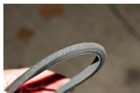
The drive belt for the water pump and the alternator (we all call it the fan belt even on a car with an electric fan!) was showing signs of decay though and was replaced.
