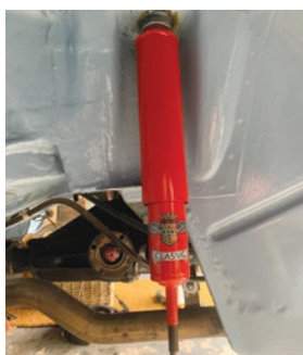
Adjustable KONI rear dampers made specifically for this application.
