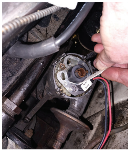
Magnetic sleeve fitted and gap checked.
