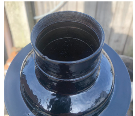
This is a refurbished strut tube with insert components removed. Note the threads at the top which must be in good condition.
