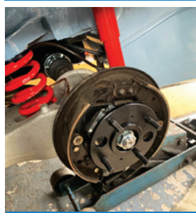
Here the CV shaft has been fitted, but not yet correctly torqued.
