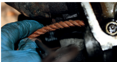
To stop the engine from turning when I tried to undo the crankshaft pulley bolt, I fed rope into No.1 cylinder. This then stopped the piston from rising.
