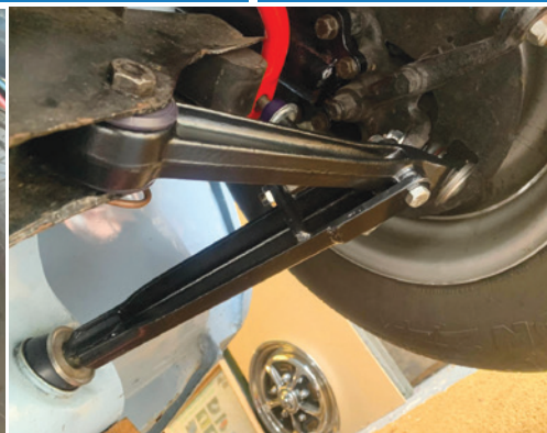
This shows the drag strut and refurbished track control arm with polyurethane bush and new quality lower ball joint.
