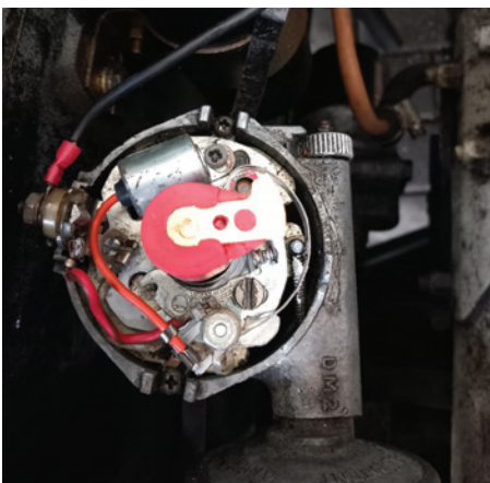
Points and condenser to be removed...
