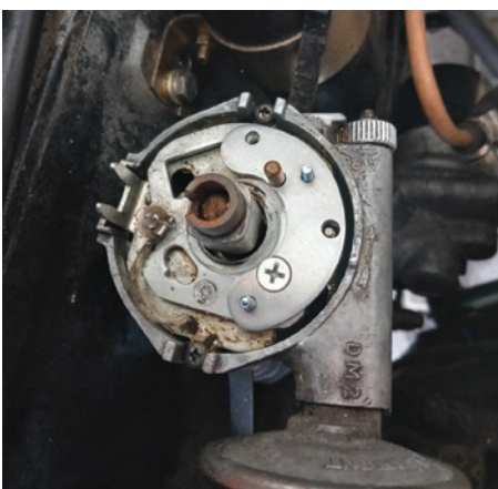
...and Igniter adaptor plate in position.
