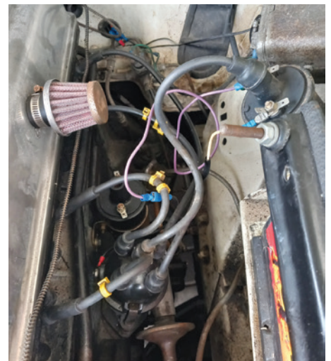
Copper HT leads must be removed...
