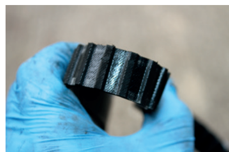
As it turned out, the old belt was unmarked and showed no sign of any cracks even when bent back on itself. It probably could have carried on for years. Probably.
