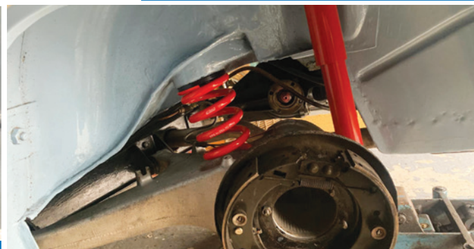
Here, new Eibach rear springs and polyurethane trailing arm bushes are added to the mix.
