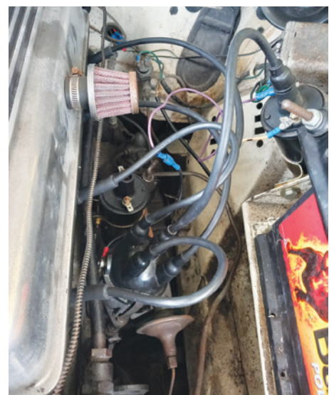
...and were replaced with new silicone HT leads.
