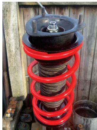
The assembled strut assembly with high quality Eibach spring, new lower powder coated top cup, Chris Witore roller bearing top mount and nut tightened to his spec.
