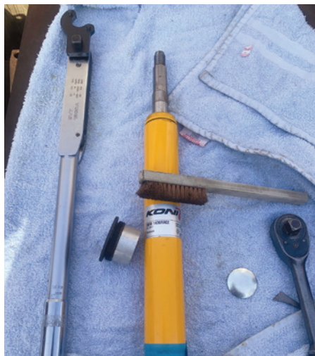
This shows the insert and spacer, and also the correct gland fitting tool on the torque wrench.
