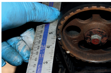
There are also two notches on the camshaft gear. They need to be positioned at 9 o'clock and 3 o'clock, in line with the top of the cylinder head.
