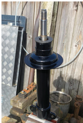
And here is the same strut with a new high quality KONI adjustable strut insert fitted.
