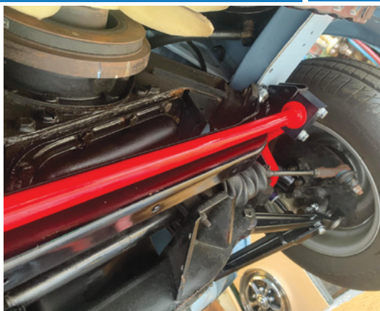
And here it is with the anti-roll bar painted red and fitted.
