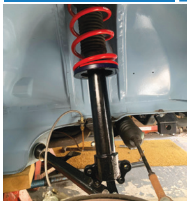
Front strut fitted – note the anti-roll bar mount and refurbished drag strut with polyurethane bushes.
