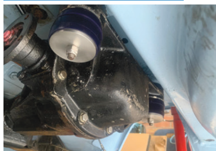
The new polyurethane diff mounts were fitted with stainless washers.
