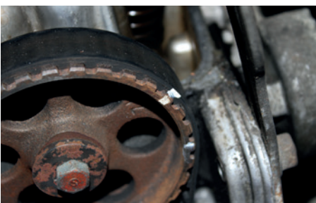
Before releasing the tensioner and removing the belt, Simon marked one tooth on each pulley and the corresponding tooth on the timing belt with Tippex.
